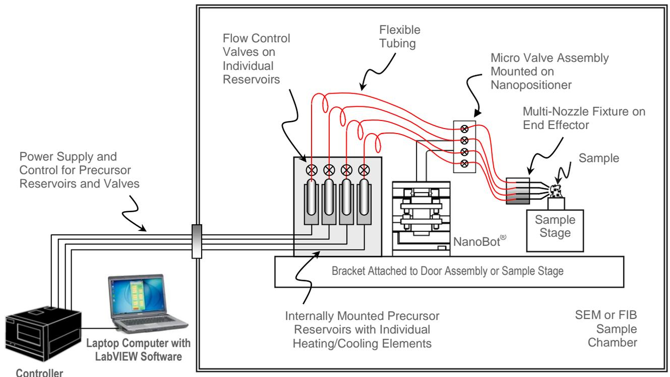
Figure 1 - Schematic of Xidex's Parallel Gas Injection System (PGIS)
